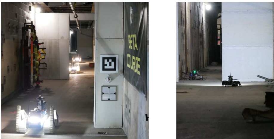
Fig. 1. Team of ground robots exploring entry hallway (left) and crashed UAV being observed by hexapod (right) during DARPA SubT at Satsop nuclear powerplant.
