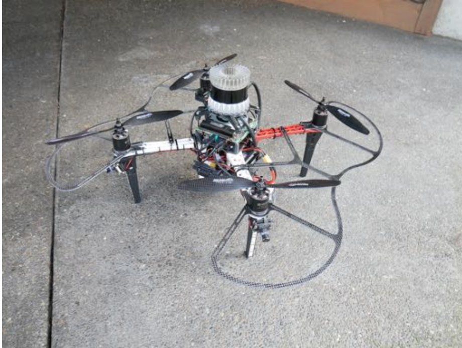
Fig. 5. One drone platform with propeler guards and Ouster sensor on top.
