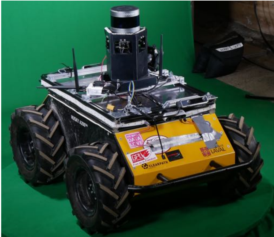
Fig. 2. The Husky platform with a Robosense lidar on top of a sensory tower which houses five cameras.
