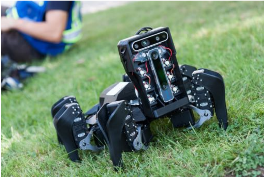
Fig. 4. Hexapod in grass “sitting” in power save mode.
