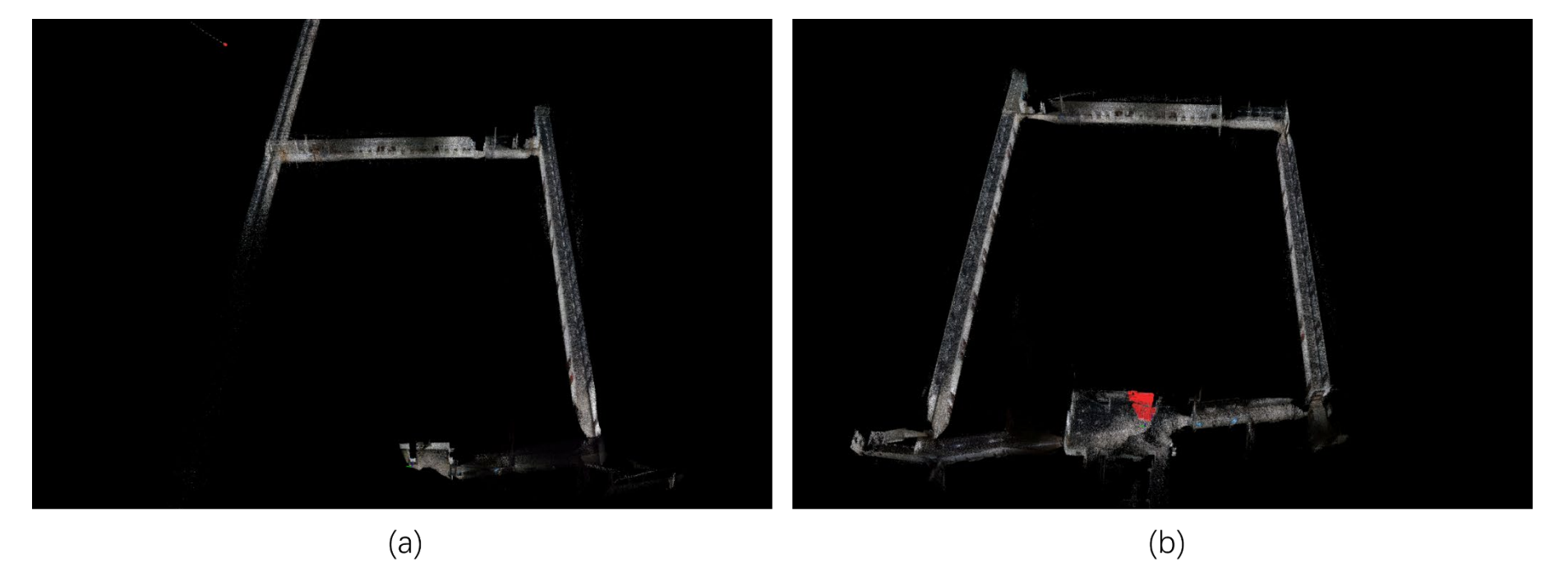
Figure 5. Comparison of mapping results between our system and Fast-LIVO2 in the Corridor01 sequence. (a) Fast-LIVO2. (b) Ours.
