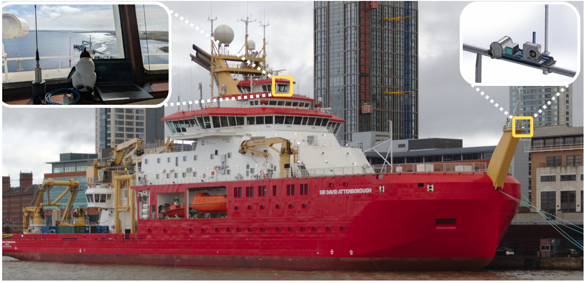
Figure 1. Shipborne multi-sensor SLAM configuration with onboard computing in the control cabin.
