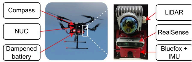
Fig. 3: Overview of the UAV platform and integrated sensor suite. The multirotor airframe carries a Livox Mid-360 LiDAR for mapping and localization, an Intel RealSense D435 depth camera for short-range obstacle perception, IMU ICM42688 coupled with VIO camera Bluefox2, and an onboard Intel NUC computer.
