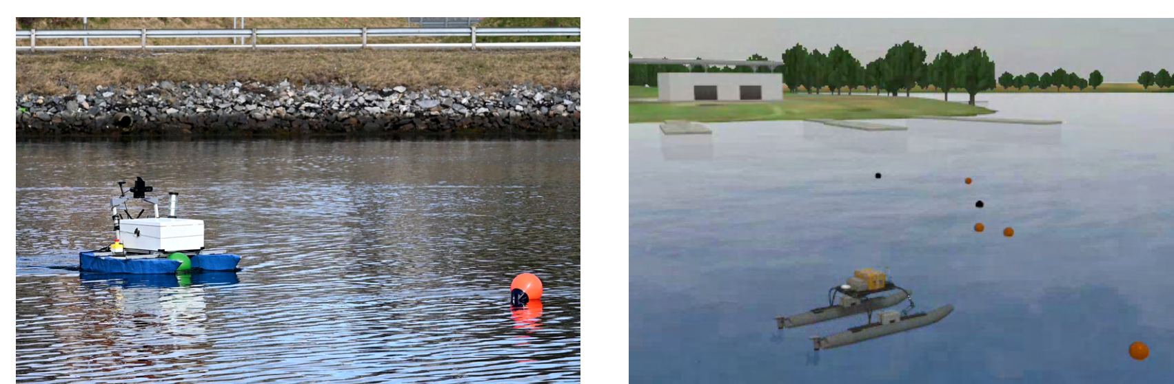
Figure: (i) Field deployment of ASV; (ii) Simulations environment for search and capture of drifting targets.
