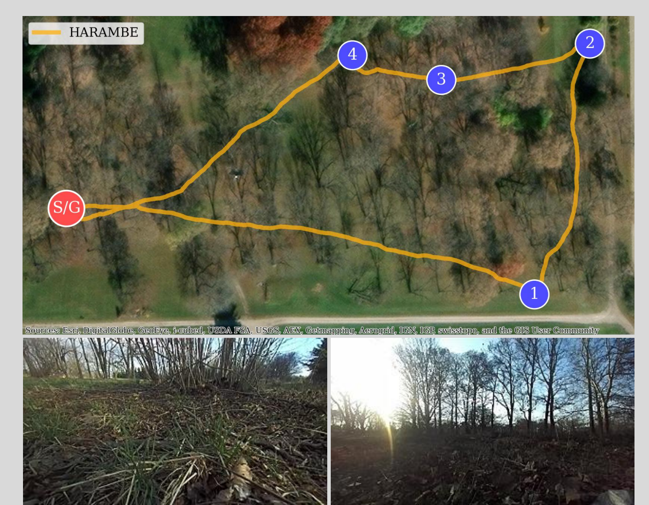
We stress test HARAMBE in a forest with obstacles and significant ground clutter (roots, leaf litter, tall grass, logs/branches, etc.), and it successfully completed a ~600 m course between 5 waypoints with no interventions. Onboard images are shown at the bottom of the figure.
